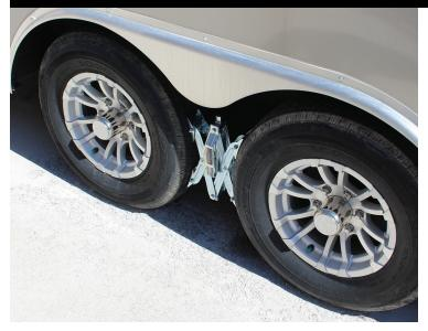
1. Use the enclosed tool to open the T-Chock to a size close to the tire spacing. Turn the middle screw clockwise to screw the chock pads into place. (**Figure 1**)
