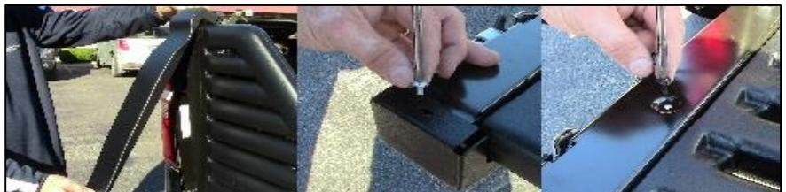
cover plate location with tape and install the screws while the gate is off your truck. Then screw through the two embosses located on the backside of the tailgate cover plate into the white blocks. Be sure not to over tighten. After installing cover plates, be sure tailgate opens and closes and lock engages and disengages properly. Before traveling, be sure center lock is in the engaged (locked) position.
