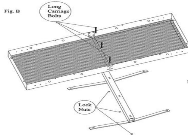
Next, use 3 long carriage bolts and 3 lock nuts to assemble platform to receiver bar and support bridges (platform assembly to items #3 & #5) (see fig B)
