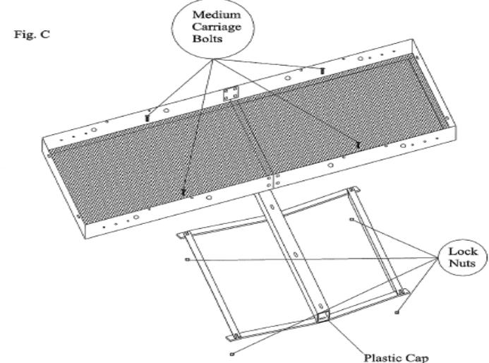
Install plastic receiver cap into open end of receiver bar that faces away from vehicle. Then install platform to your vehicle by sliding receiver tube into vehicle's receiver hitch. Clevis pin must slide through receiver hitch and receiver tube hole at the same time to secure cargo caddy properly. Place retainer clip through clevis pin.
